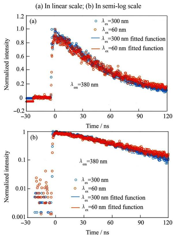
Fig. 5 Luminescence time profiles of GPS doped with Ce at 1 mol.% and La at 10 mol.%
