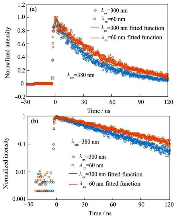
Fig. 4 Luminescence time profiles of GPS doped with Ce at 10 mol.%
