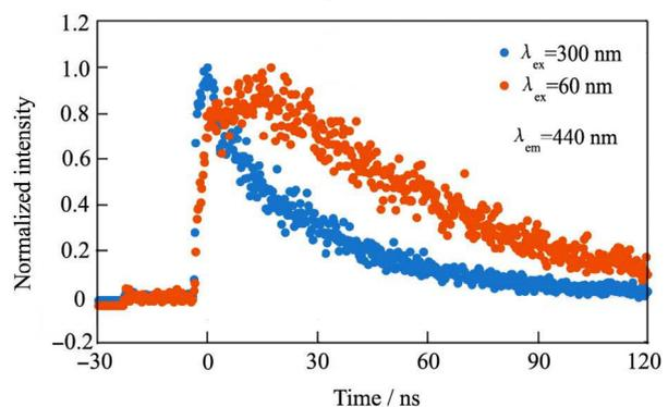
Fig. 6 Luminescence time profiles of GSO doped with Ce at 1 mol.%
